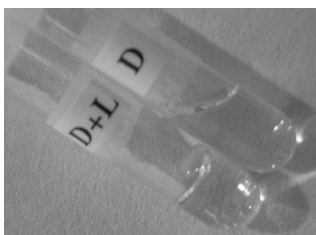
Figure 2. PDLA 15 -PEG12500-PDLA 15 13 w/v% solution (D) and PDLA 15 -PEG12500-PDLA 15 + PLLA 15 -PEG12500-PLLA 15 13 w/v% hydrogel (D+L) at room temperature.
